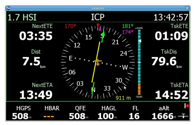
In this picture the VSI bar it is telling that we are under our planned route of more than 300 ft and that the ground is also at 300 ft (100 m) below us.
