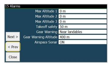
By default Sonar is enabled. The configuration choice is set on startup.
