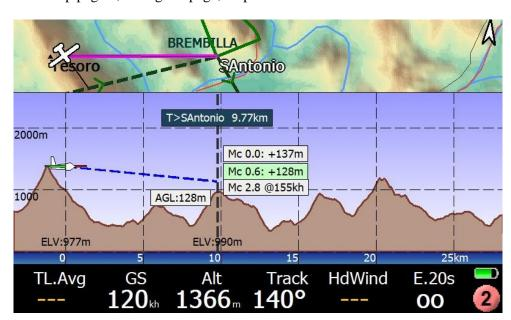
Automatically providing the minimal, current and max MC possible for the final glide, considering wind and obstacles.
